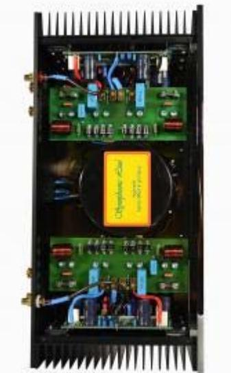
The inside leaves breathless. The symmetry is total, the logistic is witty and functional, as required for a dual mono circuit. In the middle, imposing, reign two 350 VA tower toroidal transformers, well shielded and dampening. On the left, as on the right, are two batteries with five filter capacitors each, selected to emit the same energy in all the frequencies. Altogether they are able of developing 130.000 mF of capacity: strong point!
