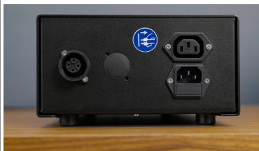
The back of the external power supply unit: The mains plug on the bottom right provides the connection to the mains socket, while the socket above it feeds the power amplifier. The four-pin socket on the left provides the necessary juice for the preamplifier.
