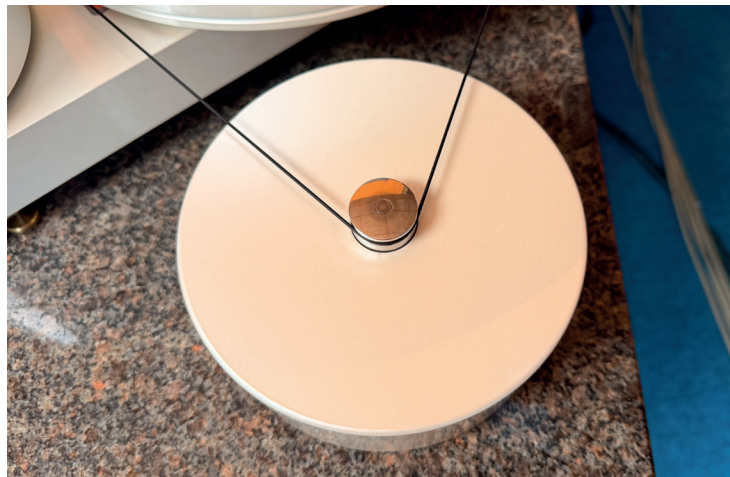
In the Reference version, the RG 6 is equipped with a second passive drive unit. It is positioned opposite the motor so that the platter is located precisely between them. This avoids one-sided tensile force on the spindle - and thus minimizes friction in the bearing.
