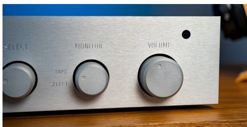
They still exist: The tape loop allows for tape monitoring when integrating a cassette deck or tape machine.
