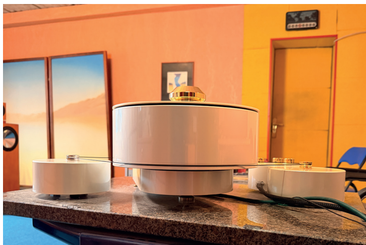
The phono cable exits from the underside of the drive chassis, allowing it to be routed discreetly. The signal cable used here is the Symphonic Line Reference NF phono cable.
